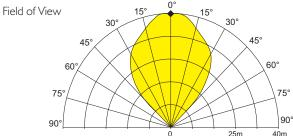
To meet the requirements of EN54:10 clause 5.4, where the ratio of the response points Dmax:Dmin should not exceed 1.41, the horizontal and vertical viewing angles  $\alpha$ max should not exceed ±30°.
